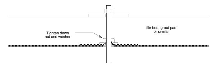
Shows the case where the device is separated from the membrane by a tile bed or similar.
