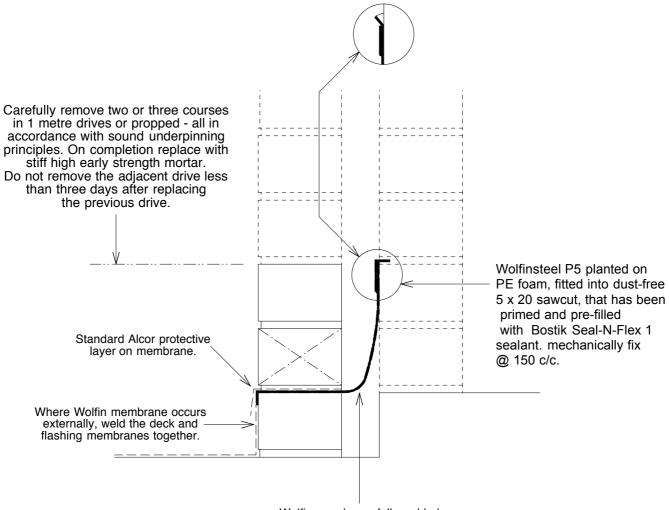
Wolfin membrane fully welded. Where the membrane is exposed to risk of mechanical damage, reinforce with a Wolfinsteel P 5 at the outer brickwork edge.
