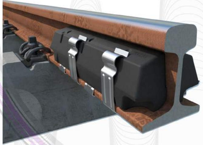
STRAILastic\_A inox 2.0 consists of a heavy, steel bar reinforced elastomer compound. The dampers are produced using a special double vulcanization process.
